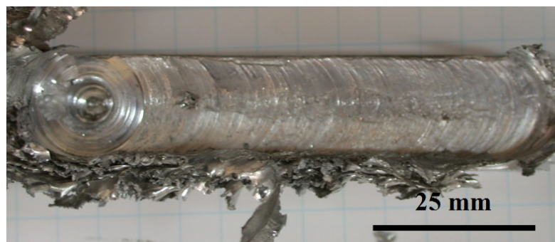
(c) \text{Mg}_{37.5}\text{Al}_{25}\text{Zn}_{37.5} material FSPed after 10 passes with copper clamping kits and water cooled
