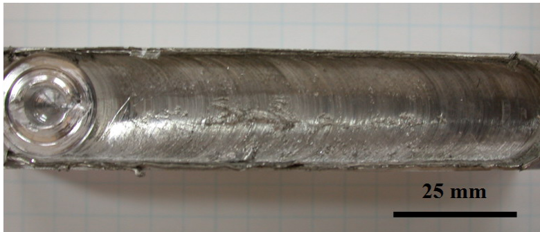
(b) \text{Mg}_{50}\text{Al}_5\text{Zn}_{45} multi-element alloy FSPed after 4 passes with 1500 rpm, 25 mm/min and 2^\circ tilt
